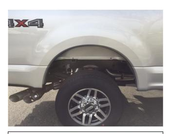
**STEP 5:** Clean the body areas where the Fender Flares will makes contact. A light misting on fender using a soap and water solution can aid in proper rubber placement.
