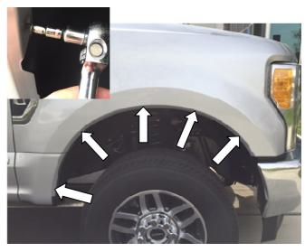
**STEP 2:** Remove all five (5) 7/32" socket head screws and retain for installation of Fender Flares.
