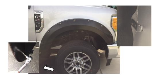
**STEP 4:** Loosely reinstall the lowest rear 7/32" socket head screws through slot in the Fender Flare to the vehicle. Make sure the screws are securely engaged to the vehicle fender. Install provided Long Attachment Clips in remaining four (4) Fender Flare Slots. Loosely reinstall remaining 7/32 in socket head screws. Ensure part is still in the position of best fit and extrusion is in correct position before hand tightening all screws.
