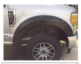
**STEP 3:** Place the Fender Flare onto the vehicle and fit into the correct position following the contours of the body. Ensure the slots in the part align with the holes in the fender from the previously removed 7/32" socket head screws.
