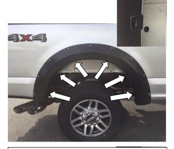
**STEP 6:** Place the Fender Flare onto the vehicle and fit into the correct position following the contours of the body. Use six (6) provided "U" Shaped Retention Clips to secure the Fender Flare to the body. Ensure the barb in the clip securely attaches in the slot on the Fender Flare. REPEAT ALL ABOVE STEPS FOR OPPOSITE SIDE OF VEHICLE.
