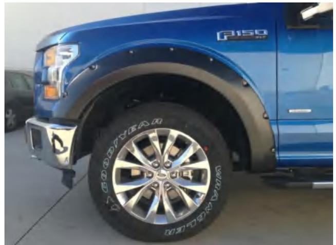
**STEP 6:** Repeat installation method for other side. Double check the front Fender Flares to make sure all bolts are tight and clips are securely fastened. Your installation is now complete. Do not use abrasive cleaners.
