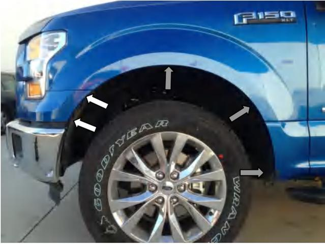
**STEP 2:** Locate three (3) 5.5mm bolts and two (2) 7mm bolt.
