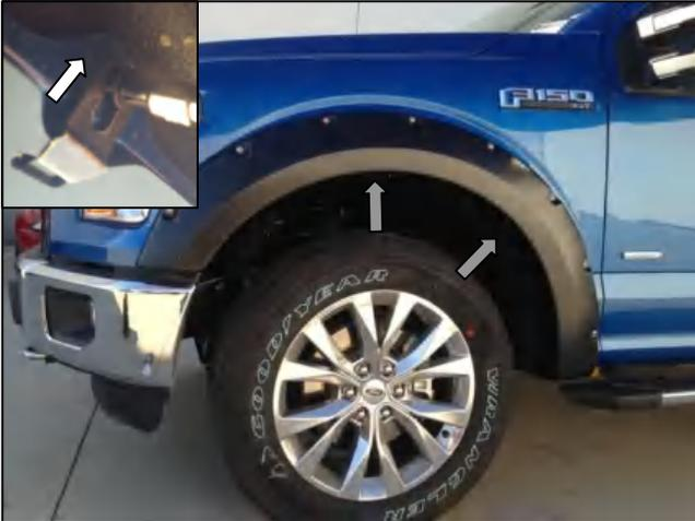
**STEP 3:** Place the Fender Flare onto the vehicle and fit into the correct position following the contours of the body. Use four (4) of the .6mm clips (two (2) per side) to secure the Fender Flare to the body. Make sure the dimple in the clip securely attaches in the slot on the Fender Flare.
