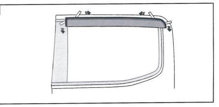
12• Using a clean, soft cloth, firmly rub down over the attachment areas 4 times to ensure maximum adhesion.
