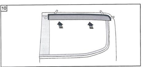
11 • Slowly peel the remaining protective tape liner away by pulling on the exposed ends of liner, and apply firm pressure around the attachment areas. 11
