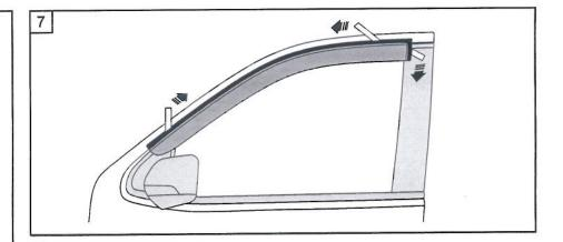
8. Using a clean, soft cloth, firmly rub down over the attachment areas 4 times to ensure maximum adhesion.
