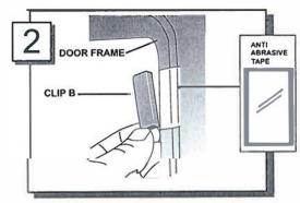
Clean the inside area of the door frame with alcohol wipe provided and wipe away any residue with a dry clean cloth. Adhere anti abrasive resistant tape to these areas. Insert the metal dip B to door frame and make sure it's resting on the abrasive resistant tape.
