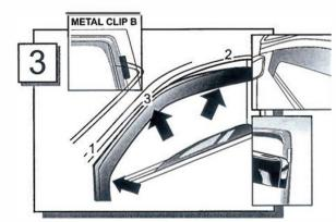
With the metal clip B in place, install WINDOW VISOR. Fit the front of WINDOW VISOR first at the mirror sail area of the door. Insert the rear of the WINDOW VISOR into the metal clip B and slide the WINDOW VISOR upwards.
