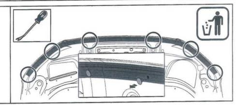
Gently peel back the rubber seal and insert a screw plug into the vacant holes in the underside of the hood.
