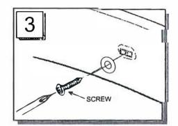
To Remove: Loosen and remove screws. Lift HOOD PRODUCT away from hood. To Clean: Use mild detergent and water solution. (Do NOT use solvents). Avoid the use of automatic "Brush Style" car washes. When closing the hood, do NOT pull on HOOD PRODUCT.
