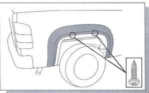
**9.** Install the black phillips head screws into the fender to secure the Fender Flares. Fit the Fender Flares loosely until the Fender Flares are aligned as desired. When satisfied, tighten the screws fully and ensure extrusion is flush neatly against the body.
