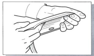
4. Remove approximately 2" (50mm) of the protective liner from the extrusion. Fit the extrusion to the Fender Flares along the edge that comes in contact with the vehicle's body panel.
