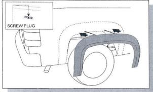
8. Place the rear Fender Flare onto the vehicle and line up the slots in the Fender Flare with those of the screw plugs on the vehicle previously installed.
