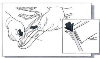
5. Pulling at right angles to the extrusion, remove the liner from the extrusion in small portions and apply thumb pressure to ensure that it adheres to the Fender Flares.
