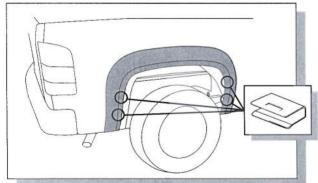
10. To secure the lower part of the Fender Flares to the body, take the black metal clips and slide them over the Fender Flares and inner wheel arch lip. Position clip so that the barb in the clip locates in the slot in the Fender Flare. Ensure all fixing points are secure and that extrusion is flush neatly against the body.
