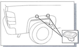
7 Take the 2 screw plugs from the hardware kit and push them into the 2 outside holes under the wheel arch on each side so they fit tightly.
