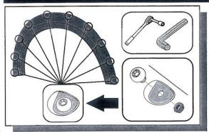
Attach 10 bolts to each Fender Flare using a 3/16" Allen key and a 1/2" wrench/socket. (socket wrench and Allen key not supplied)
