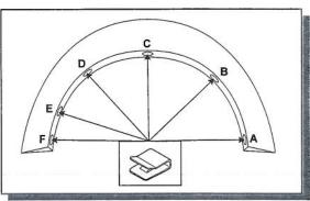
Note the correct hardware positions. (Right Fender Flare shown).
