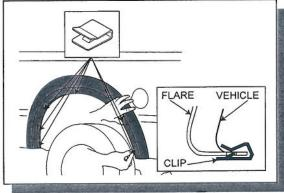
Place Fender Flare on the vehicle. Take the supplied snap clips and fix them into positions A, B, C, D, E and F, as shown, ensuring the notch in clip locates securely into the slot in the Fender Flare.
