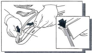
Pulling at right angles to the extrusion, remove the liner from the extrusion in small portions and apply thumb pressure to ensure that it adheres to the Fender Flares.
