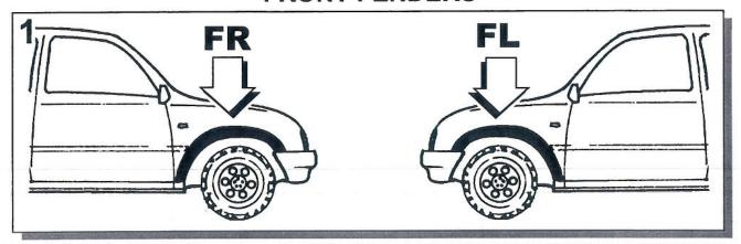
Ensure that both Left and Right hand Fender Flares suit the profile of the vehicle. Note the areas where the Fender Flares come in contact with the vehicle. NOTE: Before fitting Fender Flares remove any moldings, strips or existing flares from the wheel arch. If there is a body side moulding, mark where the moulding is to be cut. Alternatively, the Fender Flare can be cut to go around the moulding. Be sure to allow enough room for the extrusion.
