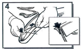
Pulling at right angles from the extrusion remove the liner from the extrusion in small portions and apply thumb pressure to ensure that it adheres to the Fender Flare.
