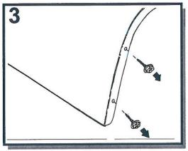
Remove the two mudflap screws as shown.
