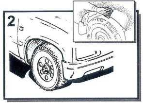
Wash the areas of contact on the vehicle and wipe dry both the vehicle and the Fender Flare with a clean cloth. Ensure inside of Fender Flare where extrusion is attached, is clean.
