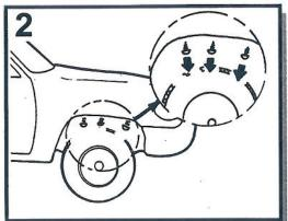
Remove the three existing screws as shown
