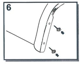
Replace the mudflap and the mudflap screws.
