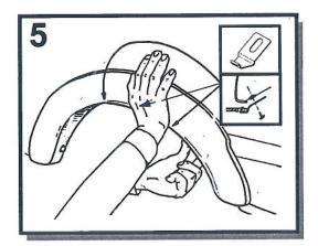
Place the Fender Flare into the position of best fit. Take three of the supplied lever clips and install them in the positions shown. Installation of these clips is achieved by removing existing screws and replacing them after the clips are positioned.
