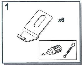
Ensure that all of the necessary hardware is in the hardware kit (screwdriver and spanner not supplied).
