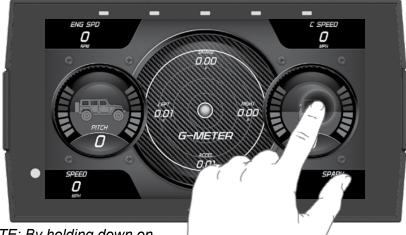
NOTE: By holding down on the pitch / roll gauge for three seconds, you can level the gauges and G-Meter out to 0.
