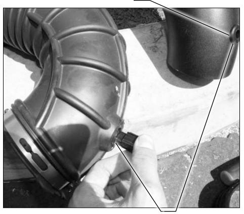
**STEP 14 -** Carefully pull the temperature sensor out of the stock intake tube. Remove the O-Ring and insert it into the grommet on your Jammer intake tube.
