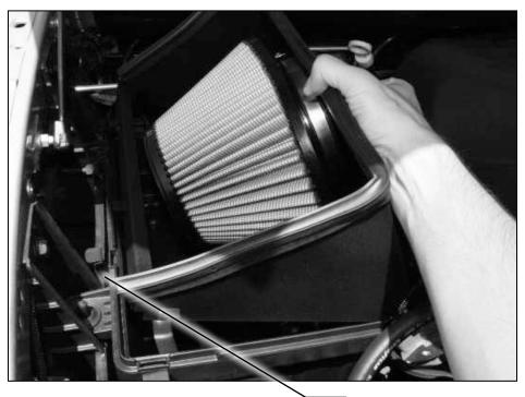
STEP 12 - Use the factory clips to secure the heat shield down onto the air box.
