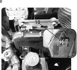
**STEP 12** - Reconnect the final blue harness connector, and after pushing down and setting in place, carefully close the clamp.
