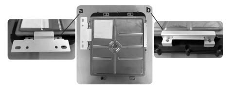
**STEP 5** - To prevent damage to the Pulsar and stock connectors, ensure that your ECM connectors and harness connectors are clean and free of debris/dirt.
