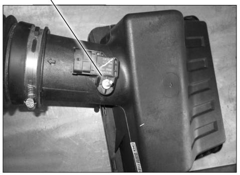
**STEP 14 -** Install the map sensor onto the Jammer intake tube using the hex head screw provided with a 10mm socket. —
