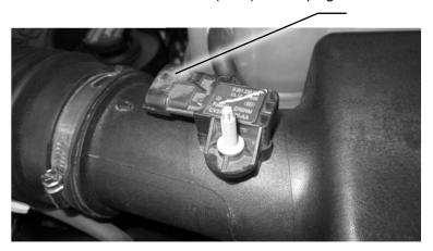
STEP 2 - Loosen the driver and passenger intake clamps.
