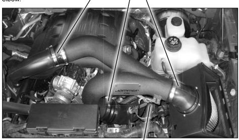
**STEP 16 -** Adjust the couplings and the tube fo/ proper alignment and then tighten all clamps.
