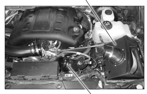
**STEP 11 -** Install the larger reduction coupling on the driver side runner. Clamp down but do not tighten.
