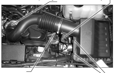
STEP 3 - Disconnect the crankcase vent tubes from the intake tube.
