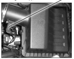
STEP 11 - Install the coupling hump and clamps on the throttle body.
