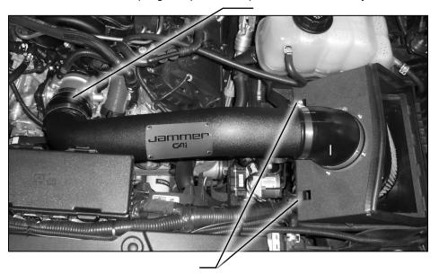
**STEP 12 -** Install the Jammer housing assembly in the lower airbox and secure using the stock front and rear clips only.
