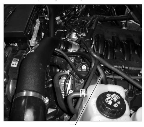
**STEP 15 -** Replace the stock crankcase vent tubes with the supplied hoses.
