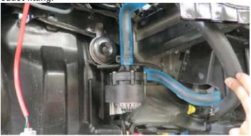
138. Route the water pump connector, from the previously installed water pump harness, down towards the water pump and connect it to the water pump. Secure the harness to existing wire looms and/or hoses.
