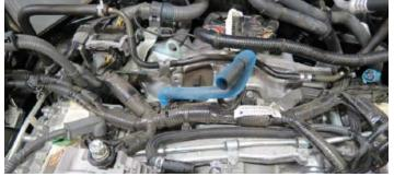
64. Install the 90° end of the supplied passenger side PCV hose onto the passenger side PCV fitting. Secure hose with a 5/8" hose clamp from Bag #4.
