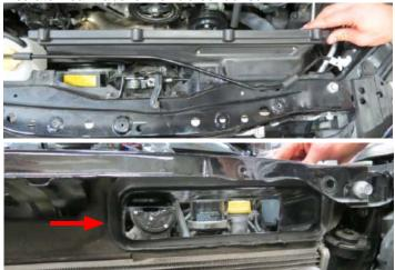
146. Use the M6 x 16mm Hex Flange bolt from Bag #4 to secure the front air box shroud to the upper radiator support. This is done from the inside of the air box by threading the bolt through the welded nut on the radiator support.
