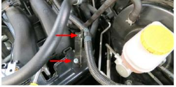
35. Using a 12mm socket, remove two (2) bolts securing the driver side manifold support bracket to the engine. *NOTE: Removal of the driver side strut brace will simplify this procedure but is not required. Reinstall the strut brace once the driver side support bracket is removed.*
