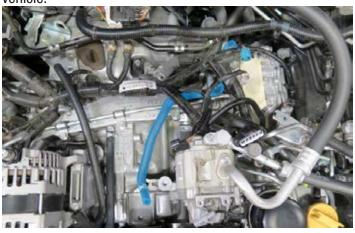
68. Using a hose clamp tool, or equivalent, remove the passenger side heater hose from the heater core fitting located on the firewall.
