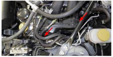
36. Carefully work the manifold support bracket towards the front of the vehicle and remove.
