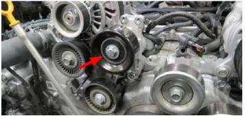
89. Rotate the tensioner clockwise using a 14mm socket and remove the small screw driver holding the tensioner open.
