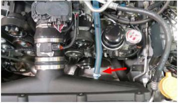
159. Using the 3/4" Hose Clamp and M5 x 8mm Button Head Flange bolt from Bag #4, secure the driver side PCV hose to the PCV support bracket.
