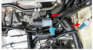
82. Using pliers, remove the factory EVAP hose from the hard line located in between the low pressure fuel feed lines.
