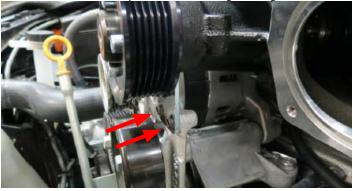
122. Connect the 45° end of the previously installed EVAP hose to the top nose fitting. Connect the RH/Passenger PCV to the bottom nose fitting. Manual applications will connect the Brake Booster hose to the center nose fitting. Automatic applications will remove the fitting plug from the stock intake manifold and install it to the center nose fitting.
