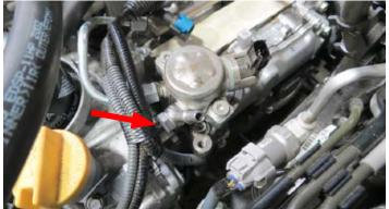
58. Install the low pressure fuel feed line onto the banjo fuel fitting. *TIP: Fuel line will be the one closest to the mechanical fuel pump.*
