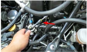
120. Reinstall the ECU mounting plate assembly using the factory hardware. Reconnect all ECU connections and reattach the engine harness and alternator harnesses to ECU plate.
