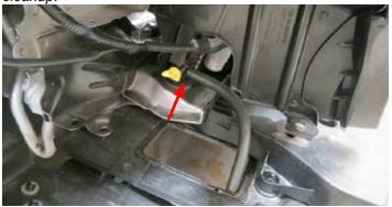
12. Using a hose clamp tool, or equivalent, remove the driver side PCV hose from the air inlet tube.
