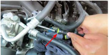
43. Using pliers, remove the rubber EVAP line from the hard line assembly.
