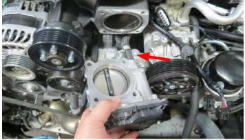
126. Using the factory throttle body bolts, secure the throttle body to the supercharger with the connector oriented upwards.
