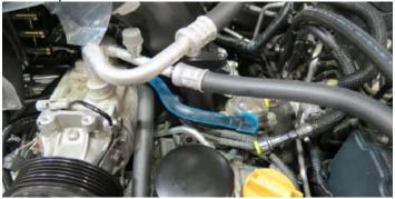
112. Realign the supercharger to the cylinder heads. Using two (2) M8 x 30mm bolts and one (1) M8 x 50 bolt, loosely secure the driver side runner to the cylinder head.
