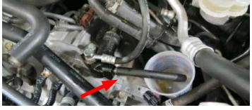
55. Using a 17mm wrench, remove the banjo bolt securing the low pressure fuel feed line to the mechanical fuel pump. Remove the fuel feed line as it will not be reused.
