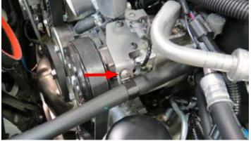
160. Connect the male MAF sensor connector, on the supplied TMAP harness, to the factory MAF sensor connector. Connect the female MAF sensor connector to the factory MAF sensor.
