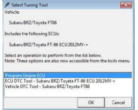
19. The ProECU Programming Tools window will only be displayed if ProECU successfully established a connection to the ECU. Proceed to Step 20 if you have established a successful connection. If not, please proceed with the cautionary notes.
