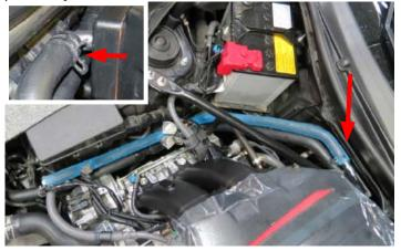
105. Attach the supplied surge tank to the other end of the Intercooler-to-Surge Tank hose and secure it with a 3/4" hose clamp from Bag #2.
