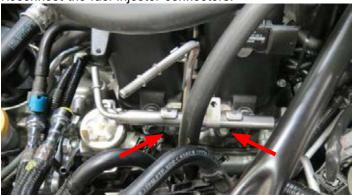
118. Connect the fuel crossover line to the driver side fuel rail and engage the blue locking clip.
