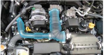
14. Using a 10mm socket, remove two (2) bolts securing the noise generator assembly to the ECU mounting plate. Disconnect the noise generator hose from the firewall and plug the hole with the 1" sheet metal plug from Bag #4.
