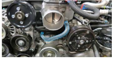
129. Using a 14mm socket, rotate the belt tensioner clockwise and install the supplied drive belt using the routing diagram below.
