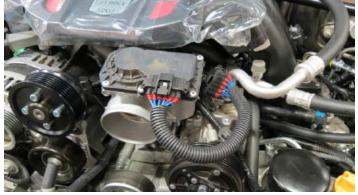
128. Using a factory hose clamp, secure the throttle body coolant outlet hose to the throttle body outlet fitting.
