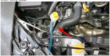
110. With the intercooler hoses properly secured, reposition the supercharger rearwards. Noting the orientation of the factory fuel crossover line, carefully snake the line under the supercharger nose, behind the alternator and out in front of the passenger side runner.
