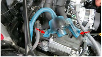
15. Remove the MAF harness from the A/C compressor pulley cover. Unplug the MAF sensor and remove it from the air box assembly using a small Phillips screwdriver. Place the MAF sensor in a clean area as it will be reused later.
