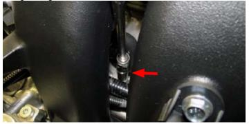
102. Position the supercharger forward to access the rear intercooler fittings. Install the straight end of the Intercooler-to-LTR Hose onto the driver side intercooler fitting and secure the hose with a 3/4" hose clamp from Bag #2. Position the 3/4" hose clamp ears away from the brake lines. Route the hose under the strut brace, in between the cylinder head and fuse box, and down towards the LTR.
