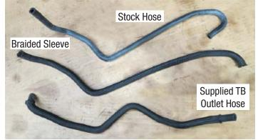
67. Install the straight end of the supplied throttle body outlet hose onto the driver side cylinder head coolant fitting and secure with a factory hose clamp. Route the hose under the engine harnesses and towards the front of the vehicle.
