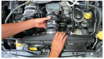
156. Clock the worm clamps to position the screws away from the A/C compressor belt/pulley. Double check that there is at least 6mm clearance between the coolant line on the throttle body and the belt on the AC compressor pulley.
