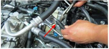
44. Using a 10mm socket, unbolt the throttle body from the intake manifold. Position the throttle body towards the front of the vehicle but do not disconnect the coolant lines at this time.
