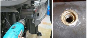
132. Secure the resistor to the rivet nut with the M5 x 20mm bolt from Bag #2. Secure the harness to existing vehicle harnesses as needed.
