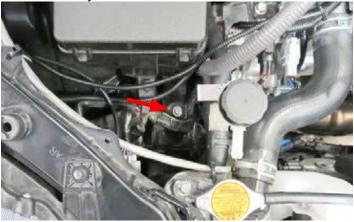
108. Using two (2) M6 x 10mm bolts from Bag #2, secure the surge tank to the surge tank bracket.
