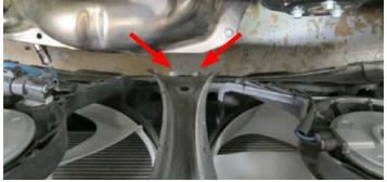
141. Install the isolator onto the lower air box support bracket. Using a 10mm socket, remove the bottom bolt securing the hood latch assembly and install the supplied lower air box support bracket using the factory bolt.
