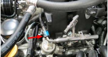
119. Connect the low pressure fuel feed line to the driver side fuel rail. Verify the lock is engaged by gently tugging on the fuel line.
