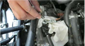
51. Remove the crush washer from the banjo bolt and from the bottom of the banjo end and discard.
