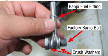
57. Carefully install the banjo fuel fitting assembly onto the mechanical fuel pump. Clock the fitting to the 1 o'clock position and torque the banjo bolt to 23 ft.lbs (31 N.m).
