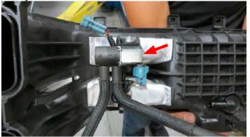
81. Secure the EVAP solenoid to the EVAP bracket using the factory nut. Connect the EVAP extension to the EVAP connector located on the water pump harness.
