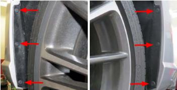
7. Carefully remove both side marker lenses by gently pulling out the upper corner of the lenses. Unplug the bulb assemblies and remove. *Tip: Lenses are secured with three (3) metal clips pointed out by the red arrows.*
