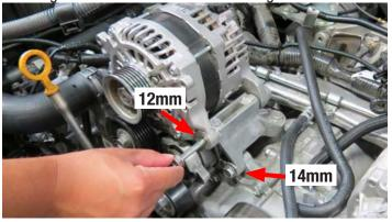
87. Position the supplied FEAD bracket onto the alternator mounting bracket. Using the M10 x 70mm bolt from Bag #1, loosely secure the FEAD bracket to the lower alternator bracket bolt provision.
