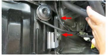
134. Using a 3/4" hose clamp from Bag #2, secure the LTR to W/P Hose to the top LTR fitting.
