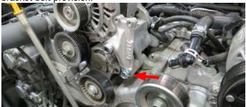
88. Using the M8 x 170mm bolt and M8 washer from Bag #1, secure the supplied pulley and the FEAD bracket to the top alternator bracket bolt provision. Torque the M8 bolt to 18 ft-lbs and the M10 bolt to 22 ft-lbs.
