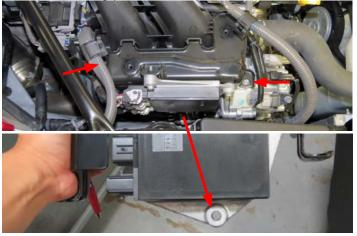
29. Place a rag under the fuel crossover line to absorb any fuel that make leak. Release the blue locking clip located on the fuel crossover line and carefully remove the fuel crossover line from the passenger side fuel rail.
