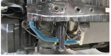
104. Install the Intercooler to Surge Tank hose onto the passenger side intercooler fitting and secure it with a 3/4" hose clamp from Bag #2. Position the 3/4" hose clamp ears away from the brake lines. Route the hose along side the previously installed intercooler hose.
