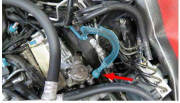
59. Using a hose clamp tool, or equivalent, remove the throttle body coolant outlet hose from the throttle body outlet fitting.
