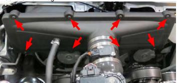
158. Connect the previously installed driver side PCV hose to the 1/2" barb fitting on the rear air box shroud.
