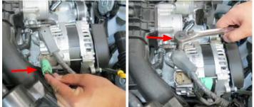
26. Remove the engine and alternator harness supports from the ECU mounting plate by pushing the locking tab in and pulling up.
