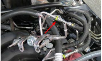
42. Using the fuel line removal tool, remove the other low pressure fuel feed line from the hard line leading to the mechanical fuel pump.
