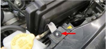
148. Use a M6 locknut and a M6 washer from Bag #4 to secure the front air box shroud to the isolator.
