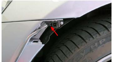
9. Unplug any front fog lights, if applicable, and carefully remove the front fascia.
