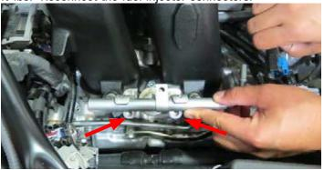
116. Connect the passenger side fuel crossover line to the fuel rail and engage the blue locking clip.
