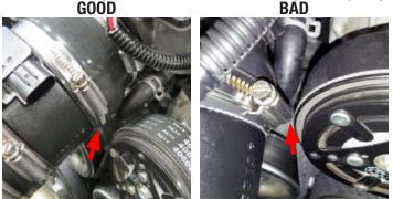
157. Secure the rear air box shroud to the front shroud using eight (8) M6 x 12mm Button Head bolts and eight (8) washers from Bag #4.
