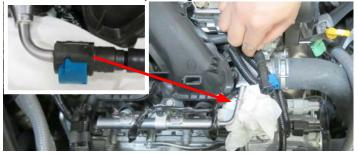
30. Remove the plastic rivet securing the fuel injector harness to the fuel rail using needle nose pliers, then unplug the passenger side fuel injector connectors. Using a 12mm socket, remove two (2) bolts securing the fuel rail to the manifold. Carefully remove the fuel rail assembly and set aside as it will be reused later.
