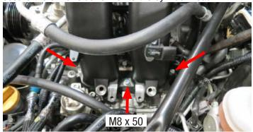
113. Using two (2) M8 x 30mm bolts and one (1) M8 x 50 bolt, loosely secure the passenger side runner to the cylinder head. Torque all six (6) bolts to 10 ft-lbs, starting with the center bolts and working outwards,
