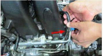
117. With the fuel injectors securely positioned on the driver side fuel rail, carefully install the fuel rail assembly with the injector connectors oriented outwards. Secure the fuel rails with the factory bolts and torque to 10 ft-lbs. Reconnect the fuel injector connectors.
