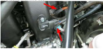
162. Using the push mount zip tie from Bag #2, secure the TMAP harness and the throttle body extension harness to the PCV support bracket.
