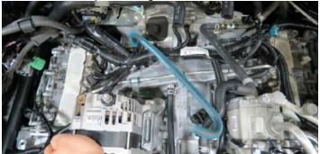
65. Using long needle nose pliers, remove the throttle body outlet coolant line from the driver side cylinder head fitting.
