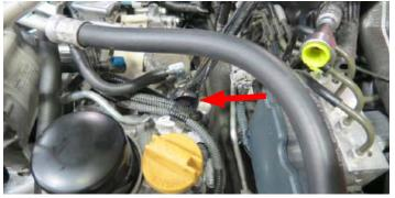
56. Assemble the supplied banjo fuel fitting from Bag #3 using the supplied 12mm crush washers and the factory banjo bolt.
