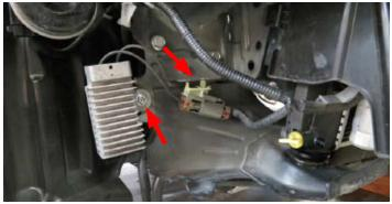
131. Using a drill and a 10mm drill bit, drill out the hole located on the crash beam support. Using a rivet nut tool, or equivalent, install the rivet nut from Bag #2 to the crash beam support.
