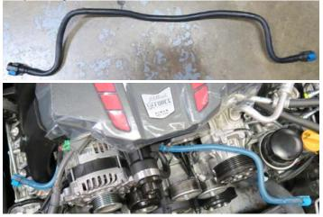
111. Snake the other end of the fuel crossover behind the A/C compressor and out in front of the driver side runner.
