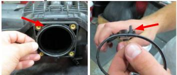
125. Install the O-ring seal onto the supercharger throttle body flange. Connect the throttle body coolant inlet hose to the inlet fitting and secure with the factory hose clamp.
