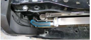
135. Route the W/P end of the hose down and over towards the water pump bracket.
