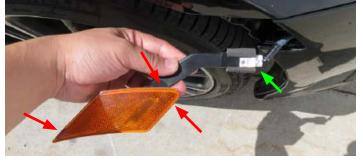
8. Using a panel puller, remove a push pin rivets securing the front fascia to the fender.
