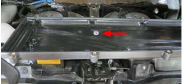
149. Re-secure the top radiator support using the factory hardware.
