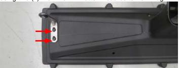
144. Install the supplied 5/16" grommet and grommet spacer onto the air duct of the front air box shroud.
