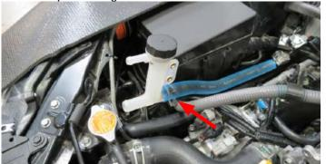
106. Using a 3/4" hose clamp from Bag #2, secure the  $90^{\circ}$  end of the Surge Tank to W/P hose onto the surge tank. Route the other end of the hose down towards the horn assembly along side the previously routed LTR hose.
