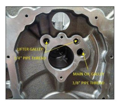
NOTE: If your engine requires an oil cooler or dry sump set up, you must install a 5/8" core plug to the bottom of the step in the red outlined oil galley located under the oil filter housing. An additional bypass is also required under the oil filter adapter as shown below.
