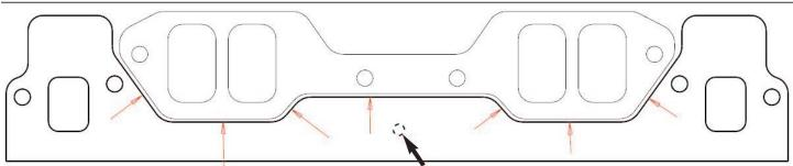
**NOTE #1:** Both intake manifolds and valley plates have been designed to fit multiple cylinder head and deck height combinations when final machining is performed to desired dimensions. Lower flange surfaces and/or the corresponding surfaces of the valley plate may require additional machining for proper manifold to valley plate clearance. This work should only be performed by a qualified engine builder or machinist.
