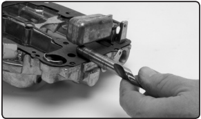
Checking float level with a 7/16" drill bit
