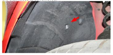
24. Reaching through the shown opening, remove four (4) nuts, two per side, securing the fascia to the fender using a 10mm socket.
