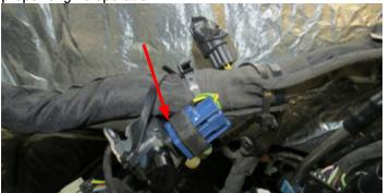
53. Tape up the end of the two (2) IMRC position sensor plugs and secure plugs to the main harness out of the way. These will not be reused.
