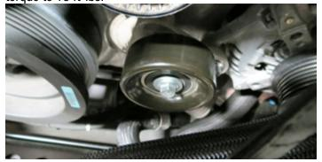
63. Verify that the tensioner is clocked correctly by sliding the index through the hole on the bracket. Install the supplied belt around the tensioner pulley and torque the M10 bolt supplied in Bag # 2 with a 15mm socket to 32 ft-lbs.
