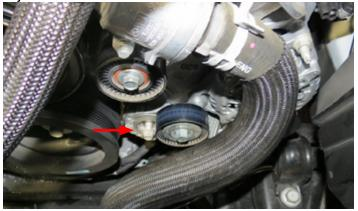
60. Remove both the engine cover bolt using a 10mm socket and the bolt through the ear of the alternator using a 15mm socket.
