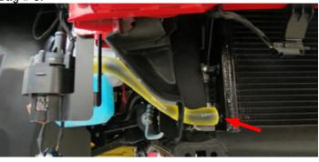
105. Insert the LTR to Manifold hose through the hole on the upper shroud and secure to the top LTR bung with a hose clamp from Bag # 3. Secure the other end to the lower bung on the supercharger manifold.
