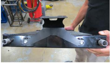
98. Back out the four (4) crash beam bolts (circled in image) but do not remove. Install the LTR assembly from under the crash beam and onto the crash beam support studs. Line up the holes on the LTR brackets with the studs to temporarily hold the LTR in place for the next step.
