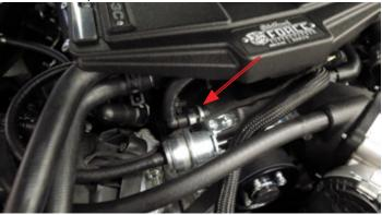
87. Remove the evap solenoid from the factory manifold. Install the solenoid onto the bracket using the factory rubber grommet. Connect the hoses. Put the evap in position and leave the bracket loose until the supercharger installation is complete.
