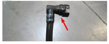
111. Attach the 90° fitting onto the supplied 1/2" Cadbar hose. Connect the quick connect fitting to the passenger side valve cover and the other end of the hose to the barb on the supercharger nose.
