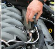
45. Disconnect eight (8) fuel injector connectors.
