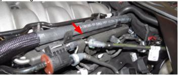
47. Repeating spill protection procedures from step 31, remove the fuel line from the passenger side fuel rail. Use a 3/8" fuel line disconnect tool to remove the line.
