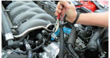
39. Remove the brake aspirator hose assembly from the brake booster and set aside as it will be reused later.
