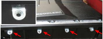
©2018 Edelbrock LLC Part #15832, 158320 71. For proper bracket alignment, test fit the side covers onto the brackets using eight (8) M6 X 25mm bolts from the side cover kit. While pushing the side covers forward, fully tighten the bracket bolts. Once all brackets are aligned and tightened, remove the side covers.
