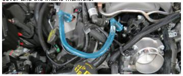
42. Disconnect the throttle body connector.
