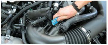
34. Remove the additional brake aspirator hose from the air inlet tube.
