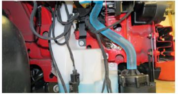
108. Secure the Surge Tank to Manifold hose to the surge tank and manifold using two (2) hose clamps from Bag # 3.
