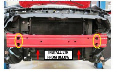
99. Install the supplied cross braces using the two (2) M8 x 30mm hex flange bolts from Bag # 3, loosely screw in the bolts through the crash beam braces. The lower cross braces will sandwich the LTR to the crash beam and be secured using the M8 nuts and washers supplied in Bag # 3. Once all bolts are in place through the braces, fully tighten the bolts and nuts.
