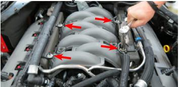
44. Remove the retaining brackets and the foam insulators from the fuel rails.
