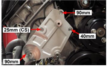
(NOTE: When installing the countersunk bolt, place the .045" thick brass spacer between the bracket and the front engine cover if the hole was drilled and tapped by the factory.) Apply blue thread lock fluid to threads and loosely install the following four (4) bolts from Bag # 2,
