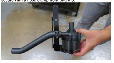
103. Feed the hose through the hole in the shroud and secure the water pump to the chassis using the supplied nuts in Bag # 3.
