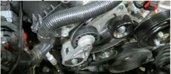
©2018 Edelbrock LLC Part #15832, 158320 64. Using the M8 x 20mm bolts and M8 washers supplied in Bag # 2, install two idler pulleys to the tensioner bracket. The top idler pulley is 65mm and the lower idler is 76mm. Add a small amount of blue thread lock fluid to the threads ONLY, do not allow excess thread lock fluid to drip onto the pulley's bearings. Torque the bolts to 18 ft-lbs.
