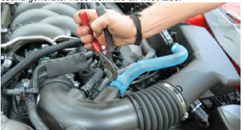
32. Remove the brake aspirator hose from the air inlet tube.
