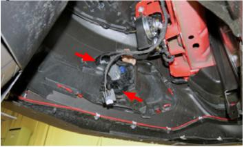
27. Tape up the fender as needed to prevent scratching the painted surfaces. With the help from an assistant, carefully disengage both sides of the fascia by gently pulling the sides outwards. Remove the fascia and set aside.
