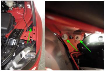
©2018 Edelbrock LLC Part #15832, 158320 25. From within the wheel well remove the fascia retention assembly that the nuts were removed from in the previous step. Pull downward until the until the plastic pin no longer retains the assembly. Remove from vehicle, ensuring to distinguish between passenger and driver side.
