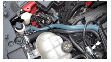
109. Using a 10mm socket, remove the top bolt securing the windshield wiper fluid reservoir. Place the surge tank bracket onto reservoir and secure the bracket and reservoir using the factory bolt.
