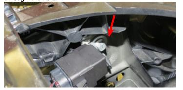
116. Route the ground strap and water pump connector downward through the frame. Remove the bolt securing the factory ground shown and mount the ground strap along with the factory ground in the original location. Connect the water pump.
