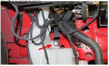
110. Using a razor blade, or equivalent, remove the 90° quick connect fitting on the factory passenger side PCV hose.
