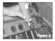
With the Edelbrock intake manifold, you must use RTV High Temp silicone sealer instead of end seal gaskets. Apply a 1/4" thick bead of sealant across each end seal surface (See Figure 5).
