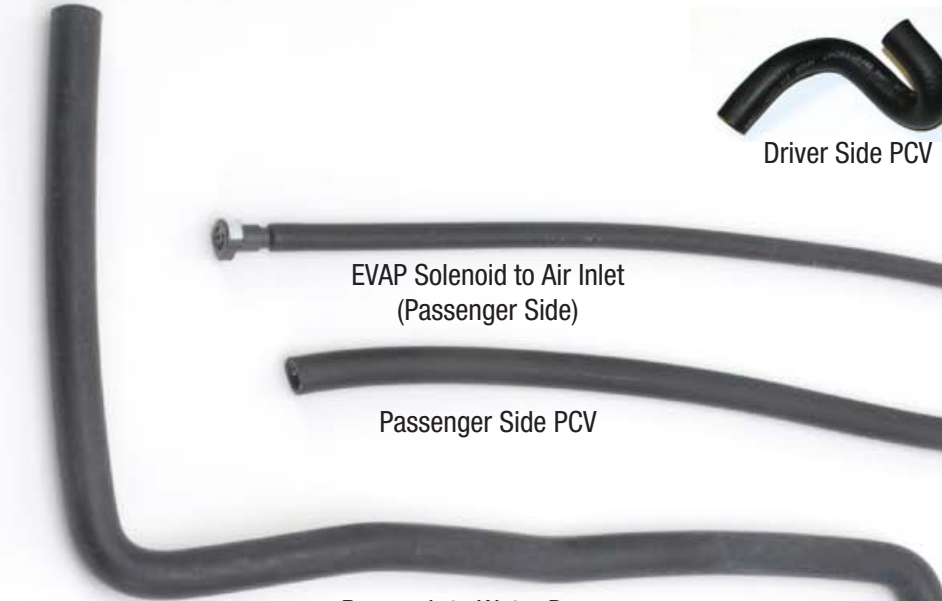
Reservoir to Water Pump
