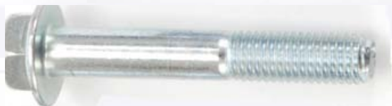
(2x) - M6 x 1.0 x 40mm Hex Flange Bolt
