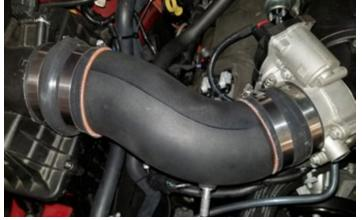
70. Reconnect the factory crank case ventilation hose to the bottom of the new intake tube.
