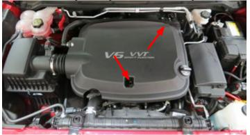
34. Using a 10mm socket, remove the bracket attaching the engine cover to the passenger side valve cover.
