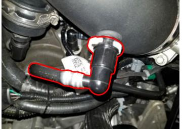
72. Unplug the MAF connector & attach the TMAP harness to the MAF. Reconnect the MAF sensor plug into the TMAP harness. Then connect the last plug into the TMAP extension located on the intake that was installed earlier.
