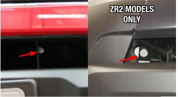
18. Using a 10mm socket, remove the bolt holding the bumper to the chassis bracket. Repeat for other side.
