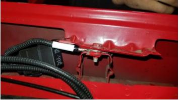
77. As you reinstall the panel, secure the relay by inserting the push-pin through the panel and then through the relay mounting tab.
