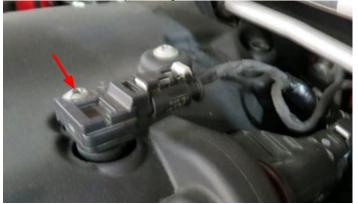
39. Disconnect the EVAP solenoid connections and then remove by using a 10mm socket as shown. This EVAP and bolt will be reused on the supercharger later.
