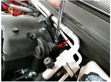
40. Using an 13mm socket and extension, loosen the 8 captive bolts holding down the intake manifold.
