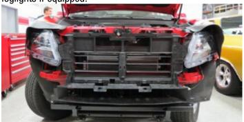
20. Remove the grill seal from the shutter assembly by removing the plastic fasteners (green arrows) and then reach inside the housing, through the shutters, and pressing the 6 tabs (red arrows) until it is free. TIP: A short flat-head screwdriver helps in disengaging the tabs. **NOTE:** Some models may not be equipped with shutters.
