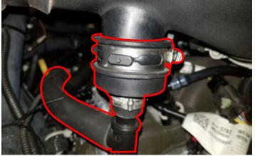
71. Connect the PCV line to the fitting on the intake tube.
