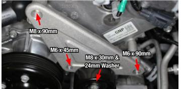
50. Attach the new vacuum pump bracket to the timing cover using the original bolt on the left side and original hardware on the right side. Reattach the pump on the new bracket and reattach all plugs and hoses.
