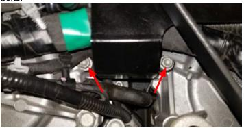
46. Using a 15mm socket, turn the tensioner counterclockwise and remove the belt from the FEAD.
