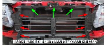
21. Using a 10mm, remove (9) bolts attaching the shutter assembly to the core support. Unplug the hood latch sensor (green arrow), unplug the shutter control cable (if equipped), and then remove the shutter assembly and set aside.
