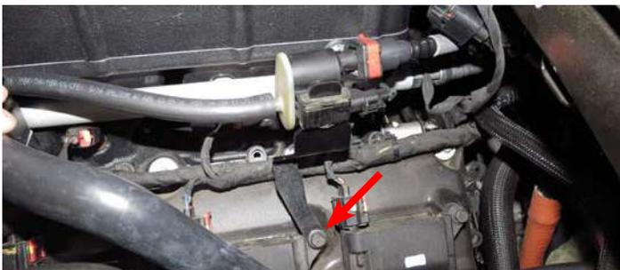
72. Attach the water pump to the water pump bracket by sliding the rubber isolator over the pump motor then onto the bracket.
