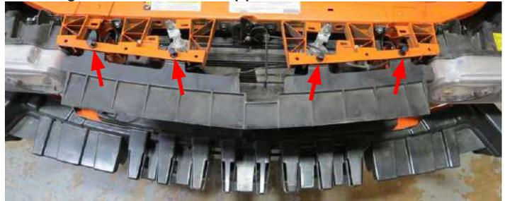
**NOTE:** Dodge Chargers and Chrysler 300s are equipped with a two piece radiator shroud. Dodge Challengers disregard step 18.
