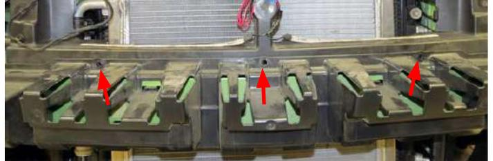
17. Using a panel puller, remove four (4) body pins securing the front fascia support and remove.
