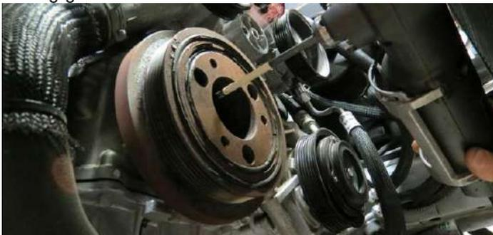
44. Use compressed air to clean out any debris present from the drilling. **CAUTION:** Use extreme caution when doing this to make sure debris does not get past the seal into the crankcase, as this will require a great deal of disassembly to correct or could cause severe engine damage if ignored.
