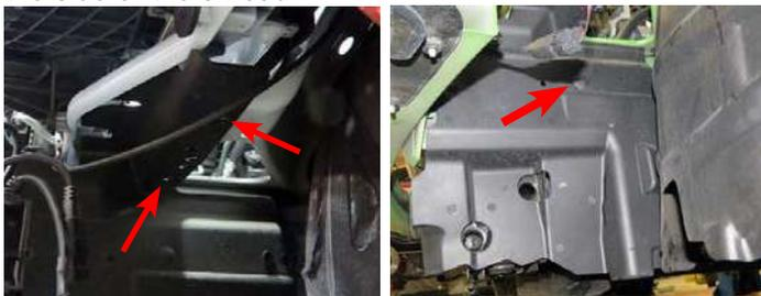
36. Using mechanic's wire or equivalent, securely hang the A/C condenser to the vehicle. Using an 8mm socket, remove four (4) bolts securing the A/C condenser to the radiator assembly.
