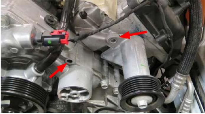
50. Using the short spacer and the bolts from Bag #2, loosely mount the idler bracket to the two bolt hole locations from the previous step. Using the long spacer and M6 x 110mm bolt from Bag #2, secure the bracket to the third bolt location; the provision on the cylinder head above the idler pulley bolt removed from Step 49. Torque all bolts to 21 ft/lbs.
