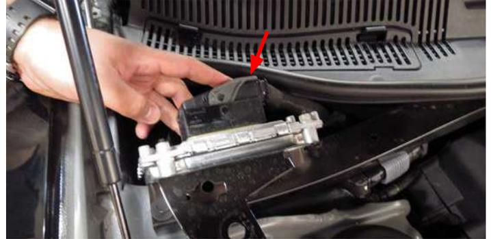
5. Using a 10mm socket, remove the two (2) nuts securing the mounting bracket to the ECM.
