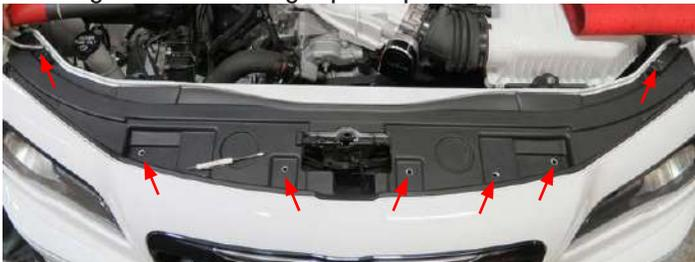
10. Use a 10mm universal socket to remove the bolts at both top corners of the front fascia.
