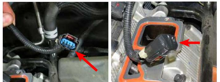
32. Using a 10mm socket, remove two (2) bolts securing each ignition coil. Remove the coils and note their order so that they can be reinstalled in the same order.
