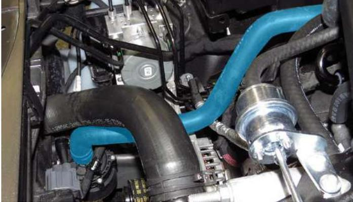
84. Install the Manifold to Tank hose between the supercharger and tank. Secure both ends of the hose with hose clamps from Bag #3.
