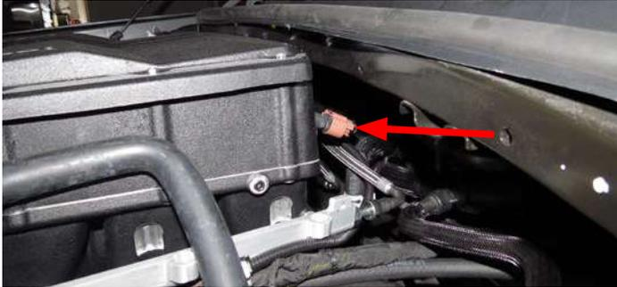
94. Connect the IAT extension harness to the stock IAT connector. Route the IAT extension harness behind the manifold and connect to the IAT sensor located on the rear passenger side of the manifold.
