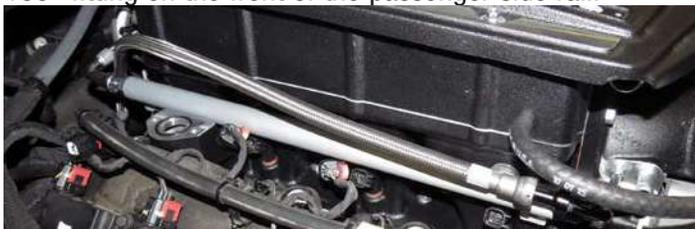
66. Using a 10mm socket, secure the fuel rails to the manifold using four (4) M6 x 40mm bolts supplied in Bag #1. Remove the oil fill cap from the stock intake manifold and install it on the supercharger. Reconnect all eight (8) fuel injector connectors.
