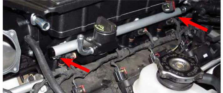
67. Attach the supplied brake booster hose to the check valve and route the hose to the driver side air inlet located on the supercharger snout.
