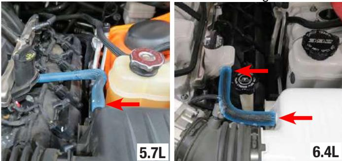
22. Loosen the worm clamps securing the air inlet tube to the airbox and throttle body. Disconnect the engine harness from the IAT sensor and remove the air inlet tube. Using a 8mm socket, remove the bolt securing the stock airbox and remove the airbox.
