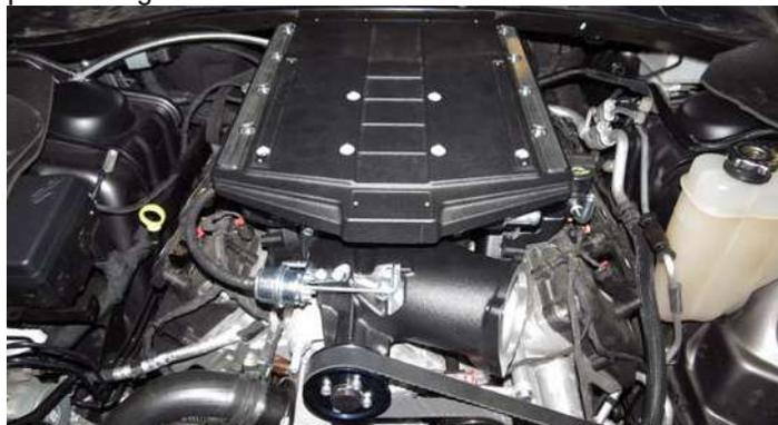
59. Use a 10mm universal socket to install eight (8) M6 x 30mm intake manifold bolts from Bag #1 following the sequence shown below. Torque all bolts to 8 ft-lbs in the same order.
