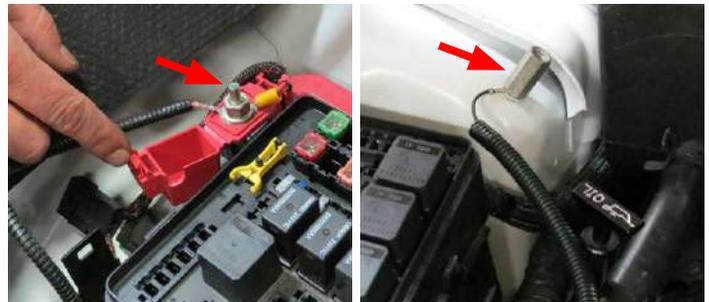
99. Feed the fuse tap wire on the Water Pump harness through the opening of the fuse box as shown. Using crimpers, connect the fuse tap wire to the butt connector installed on the fuse tap.
