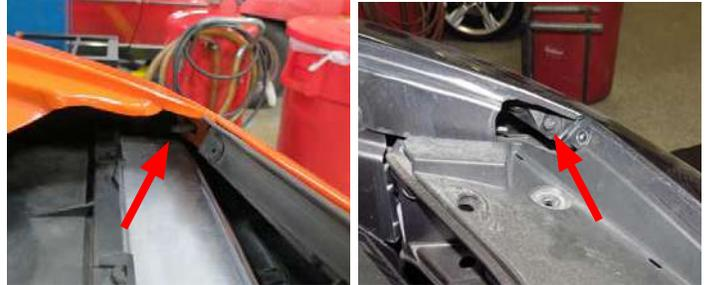
11. Use a panel puller to remove body pins securing the wheel well to the front fascia. Some vehicles use plastic rivets that need to be cut for removal. Pins are provided for reinstallation later.
