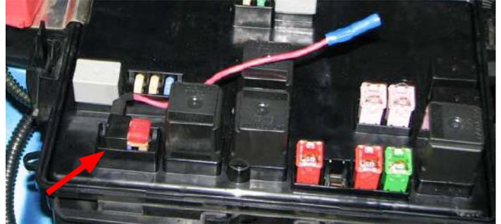
96. Use a 1/8" drill bit to drill a hole in the plastic rivet closest to the passenger side strut tower. Feed the bare wire extending from the water pump harness through the hole and insert it into the butt connector on the fuse tap. Crimp the butt connector firmly to secure the connection.
