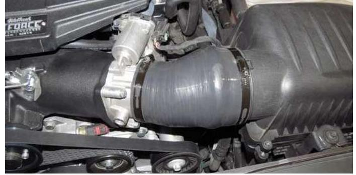
**6.4L Engines:** Use the factory rubber elbow and clamps. **NOTE:** The IAT sensor should be removed and the hole plugged with the included plastic plug.
