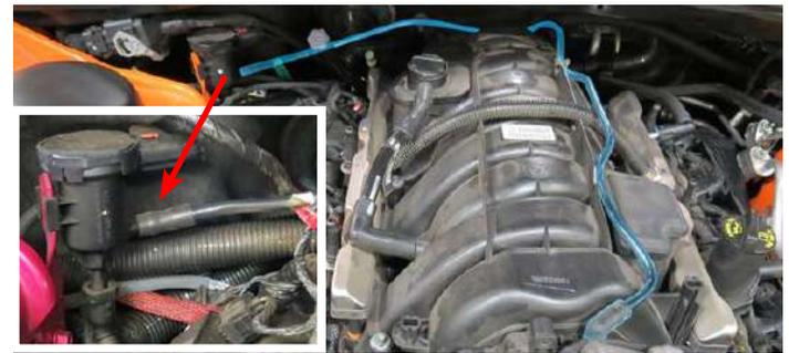
24. Disconnect the electric throttle control connector from the throttle body.
