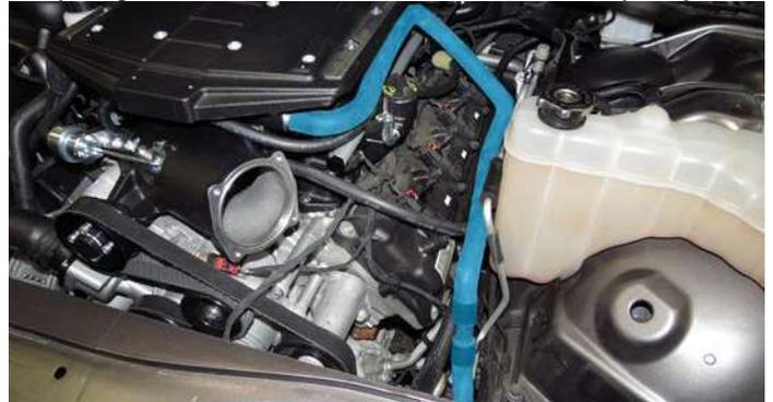
87. Attach the LTR to Manifold hose to the LTR and secure with a hose clamp from Bag #3. Apply two (2) pieces of convolute sleeve, about three (3) inches each, to the LTR hose as shown and secure with electrical tape or equivalent.
