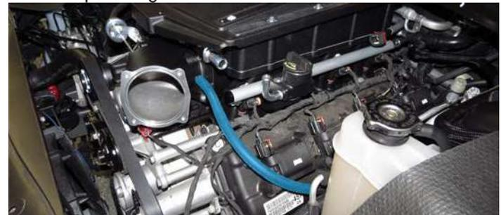
68. Attach the supplied passenger side PCV hose to the front fitting on the passenger side of the air inlet and then to the PCV fitting as shown.
