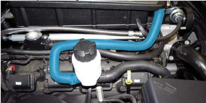
85. Connect the previously install Water Pump to LTR hose to the LTR and secure with a hose clamp from Bag #3. Apply six (6) inches of convolute sleeve to the LTR hose and secure with electrical tape or equivalent.
