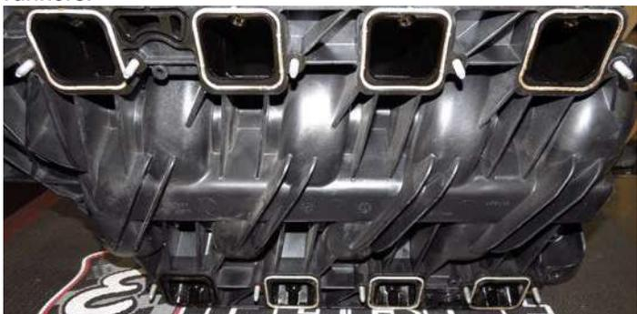
58. With the help of an assistant or a cherry picker, lift the supercharger into the engine bay. Use the intake bolt holes and injector bores to achieve the best alignment possible between the engine and the supercharger. **NOTE:** Ensure that all eight (8) O-ring gaskets are in place before proceeding.
