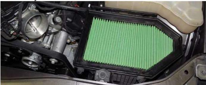
91. **5.7L Engines:** Install the provided silicone elbow onto the throttle body and the airbox lid. Secure with the provided worm clamps. **NOTE:** The silicone elbow should be loosely installed before securing the airbox lid to the lower half.
