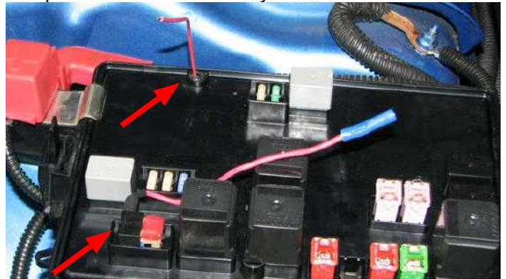
97. Tilt the fuse box up and remove the right nut. Mount the water pump harness relay on the protruding stud and reinstall the nut. Proceed to Step 100.
