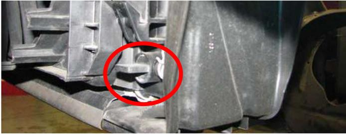
21. Remove the driver side PCV hose. Note that the 5.7L and 6.4L have different driver side PCV configurations.
