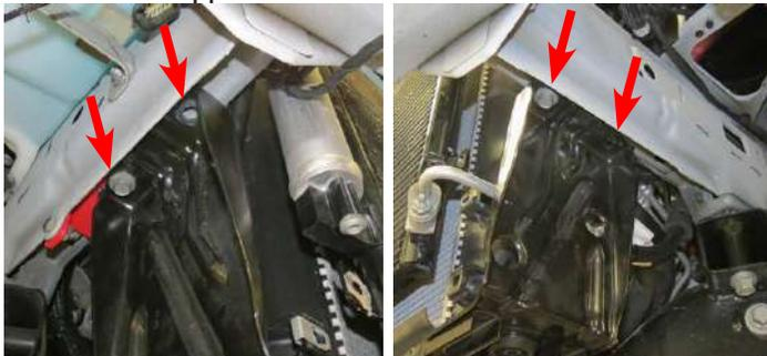
78. Using side cutters or equivalent, cut off the condenser support cables installed earlier.
