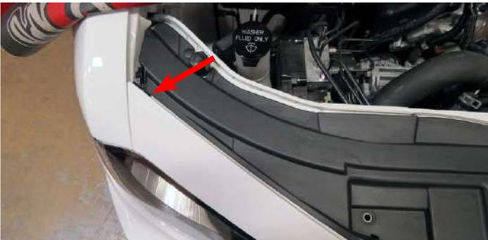
15. Unplug the ambient temperature sensor and detach the harness from the radiator shroud using a panel puller to remove the panel pin.
