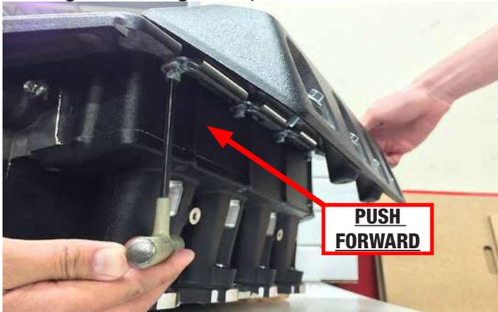
57. Remove the tape covering the intake ports of the heads and inspect the area to ensure that no residue remains on the flanges. Remove the plastic film from the supercharger ports if not already done so. Transfer the factory intake manifold gaskets to the supercharger runners.
