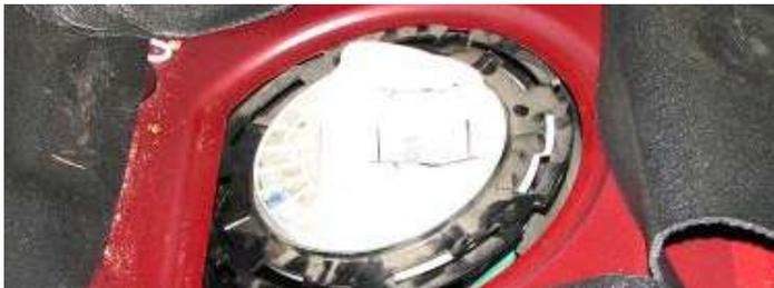
121. Lift the fuel pump module up to access the lower power connections. Disconnect the connectors from under the top of the fuel pump module and set aside.
