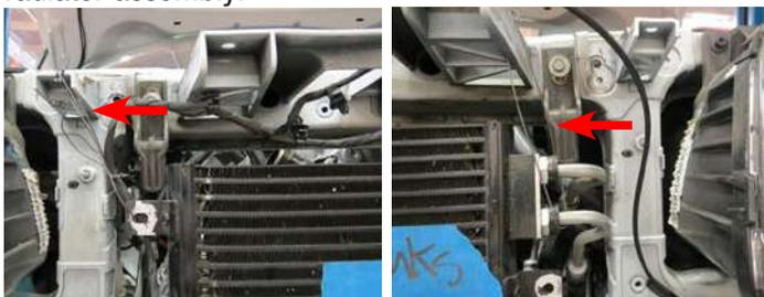
37. Remove all radiator hoses from the radiator if not already done so. Remove the fan harness and clip from the radiator assembly. Using a 13mm socket, unbolt the radiator support brace.
