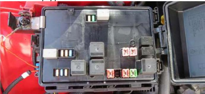
95. Open the fuse box and remove the fuse from location 6 (Ignition Coils/Injection 25A - See reverse of fuse box cover), this will be the front most fuse on most applications. Install that fuse in the bottom slot of the supplied fuse tap and the supplied 10 amp fuse in the top slot. Install the fuse tap in the slot previously occupied by the stock fuse.
