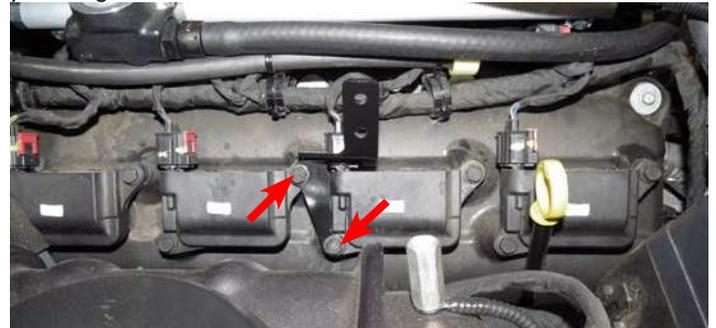
82. Attach the intercooler reservoir to the supplied bracket using the two M6 x 10mm bolts supplied in Bag #3.
