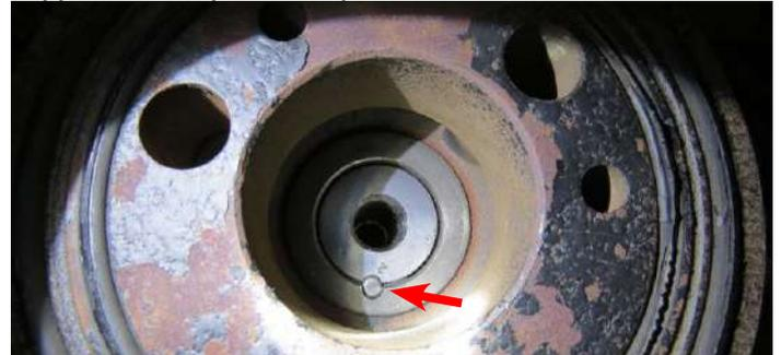
47. Using a 21mm socket, reinstall the factory crank bolt and torque to 127 ft/lbs. Remove the tool used to jam the flywheel and reinstall the dust cover if applicable.
