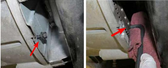
42. Using a 21mm socket and breaker bar, remove the factory crank bolt. Using the supplied crank bolt, install the drilling guide with the flat side facing outwards. Position drilling bushing in a comfortable position for drilling.
