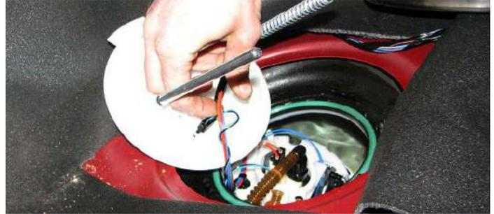
122. Press the quick connect release tab on the fuel supply line and remove. Now, disconnect the lower fuel pump module electrical connector and fuel return lines.
