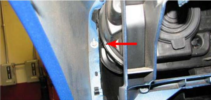
14. Carefully detach the sides of the front fascia and remove. Chrysler vehicles must also detach the top corners of the fascia.
