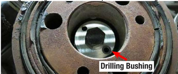
43. Mark the supplied drill bit 1.3" from the end of the tip with masking tape. Using the drilling bushing as a guide, drill into crank until the tape mark on the drill bit meets the drilling guide.
