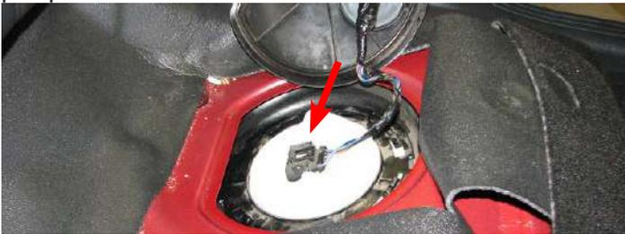
**NOTE:** Prior to removing the fuel pump module, remove any dirt or debris around the fuel tank opening with compressed air or shop vac.
