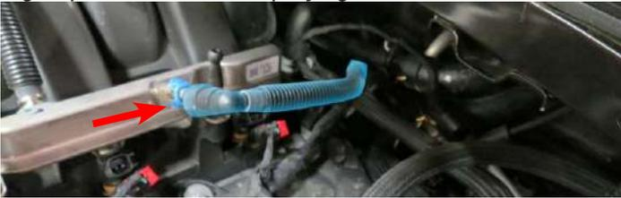
26. Unplug all eight (8) fuel injector connectors. Then use an 8mm socket to remove the ten (10) manifold bolts.
