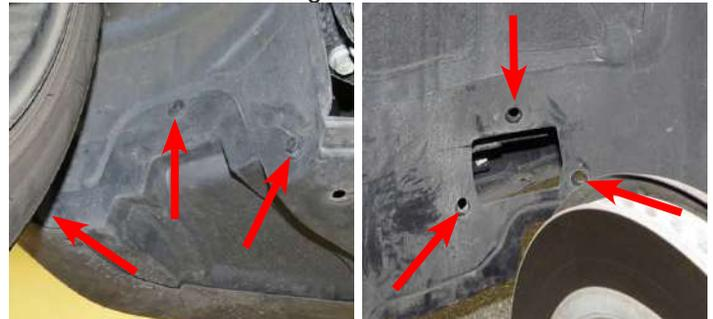
6. Using a 7mm socket, remove the nine (9) bolts retaining the splash shield to the front lip. Some vehicles are equipped with only seven (7) retaining bolts.
