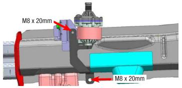
74. **2015+ Model Year Chargers Only:** Using the factory hardware, replace the existing bracket located under the passenger side headlight with the provided bracket to allow sufficient clearance for intercooler hoses.
