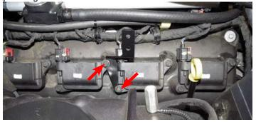
82. Attach the intercooler reservoir to the supplied bracket using the two M6 x 10mm bolts supplied in Bag #3.
