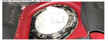
121. Lift the fuel pump module up to access the lower power connections. Disconnect the connectors from under the top of the fuel pump module and set aside.
