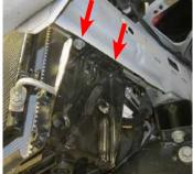
78. Using side cutters or equivalent, cut off the condenser support cables installed earlier.
