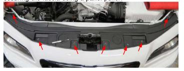
10. Use a 10mm universal socket to remove the bolts at both top corners of the front fascia.
