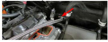
55. Apply blue thread lock fluid onto the threads of the eight (8) M6 x 12mm SHCS bolts from the side cover kit and loosely screw on the side cover brackets to the underside of the supercharger lid.
