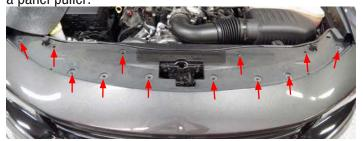
Chrysler vehicles need to remove seven (7) body pins securing the fascia using a panel puller.
