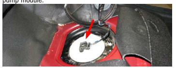
**NOTE:** Prior to removing the fuel pump module, remove any dirt or debris around the fuel tank opening with compressed air or shop vac.
