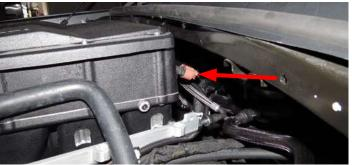
94. Connect the IAT extension harness to the stock IAT connector. Route the IAT extension harness behind the manifold and connect to the IAT sensor located on the rear reconnect side of the manifold.
