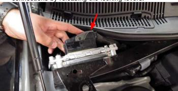
5. Using a 10mm socket, remove the two (2) nuts securing the mounting bracket to the ECM.
