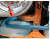
76. For vehicles equipped with an oil cooler, install the supplied thermostat housing and trim off the highlighted portion of the hose shown below. Secure the hose to the new housing with the factory clamp.
