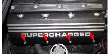
117. Using the eight (8) M6 x 25mm bolts from the side cover kit, secure the side covers to the brackets previously installed during steps 55 & 56.
