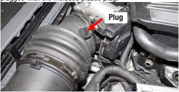
92. Install the driver side PCV hose onto the fitting next to the oil fill cap and then to the PCV fitting on the airbox. Be sure the hose does not kink.
