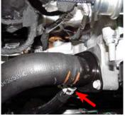
77. Reinstall the radiator assembly using the factory bolts. Reinstall the upper and lower radiator hoses.
