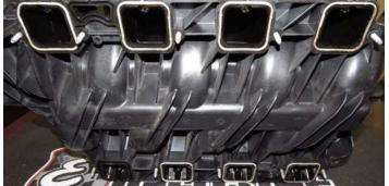
58. With the help of an assistant or a cherry picker, lift the supercharger into the engine bay. Use the intake bolt holes and injector bores to achieve the best alignment possible between the engine and the supercharger. **NOTE:** Ensure that all eight (8) O-ring gaskets are in place before proceeding.
