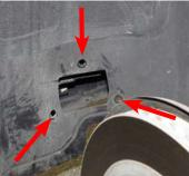
6. Using a 7mm socket, remove the nine (9) bolts retaining the splash shield to the front lip. Some vehicles are equipped with only seven (7) retaining bolts.
