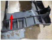
109. Reinstall the front fascia support and the front bumper absorber using the factory hardware.
