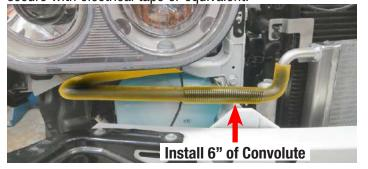
86. Install the LTR to Manifold hose onto the driver side intercooler fitting and secure with a hose clamp from Bag #3. Route the hose down towards the LTR making sure the hose is routed under the A/C lines as shown. *NOTE:* Use caution when routing the hose to ensure it will not contact sharp edges, the exhaust manifold or drive belt pulleys.
