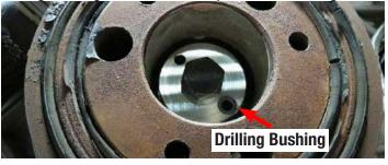
43. Mark the supplied drill bit 1.3" from the end of the tip with masking tape. Using the drilling bushing as a guide, drill into crank until the tape mark on the drill bit meets the drilling guide.
