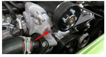
105. Vehicles with power steering cooler that installed an extension hose should check fluid levels and refill if necessary.
