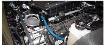
68. Attach the supplied passenger side PCV hose to the front fitting on the passenger side of the air inlet and then to the PCV fitting as shown.
