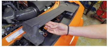
9. Dodge vehicles need to remove twelve (12) body pins, under the plastic radiator shroud, securing the fascia using a panel puller.
