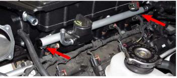
67. Attach the supplied brake booster hose to the check valve and route the hose to the driver side air inlet located on the supercharger snout.
