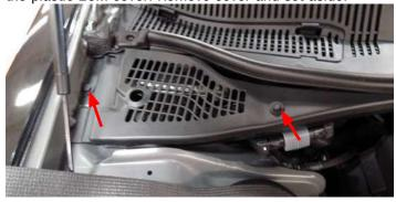
Dodge Charger/Chrysler 300: Using a panel puller, remove the five (5) push pins securing the passenger side of the plastic cowl.
