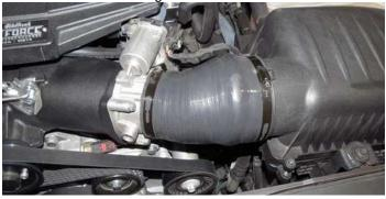
**6.4L Engines:** Use the factory rubber elbow and clamps. **NOTE:** The IAT sensor should be removed and the hole plugged with the included plastic plug.
