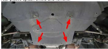
5. Using a panel puller, remove six (6) body pins from the front splash shield. Some vehicles are equipped with ten (10) body pins. If equipped, remove the three (3) screws attached to the air ducting on each side of the vehicle.
