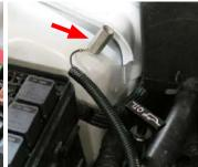
103. Remove the intercooler reservoir cap and fill the system with a 50/50 blend of water and antifreeze. Please refer to "How to Prime the Edelbrock E-Force Intercooler System" on page #28.
