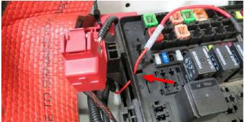
100. Mount the relay and fuse holder on the water pump harness on the metal tab with a wire tie.
