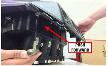
57. Remove the tape covering the intake ports of the heads and inspect the area to ensure that no residue remains on the flanges. Remove the plastic film from the supercharger ports if not already done so. Transfer the factory intake manifold gaskets to the supercharger runners.
