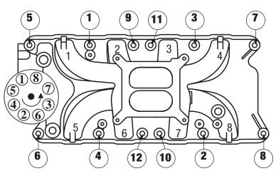
Figure 2 - 260-289-302 Ford Torque Sequence
