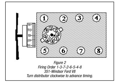
CAMSHAFT: Performer-Plus Hydraulic CATALOG #2182 ENGINE: Ford 351-Windsor V8 RPM RANGE: Idle-5500 CAUTION: Do not use dual valve springs. Use only recommended stock or Edelbrock Sure Seat Valve Springs #5882 or #5982 Use stock ratio rocker arms only.
