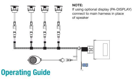
System will become engaged when vehicle is put into reverse. The system should beep one time when reverse is activated to notify the driver that it is on and working. Once an object is detected within the range, the system will alert the driver via audible tone or visual indicator (if using the display).
