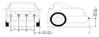
Sensor Install: Sensors must be installed in order 1-4 from left to right with control module harness entering trunk near sensor #4. If only using 2 sensors for the install, it is recommended to use sensors 2 and 3.
