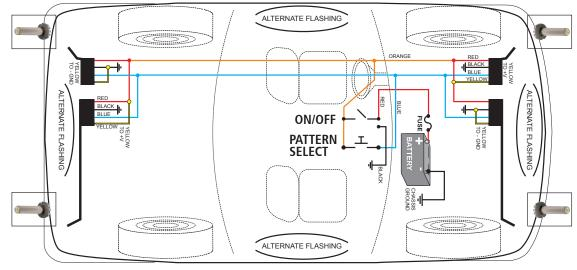
The front and rear heads are configured to flash independently of each other. In order to have the front and rear heads flash in sychronization, the blue wires from all units must be connected. The yellow wire can then be used to determine either alternate or simultaneous flash between each unit in the system by connecting to either power or ground.
