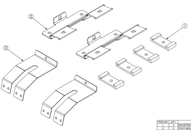
DESCRIPTION COMMENTS MOUNTING PAD, RUBBER, LIGHT BAR FOOT, MOUNTING STRAP,FORD TRUCK,SD,2010 SHEET, INSTRUCTION, STRAP, TRILINGUAL NOT SHOWN 5 BOX,ACCESSORY,CRAFT NOT SHOWN 6 BAG,POLY,8 X 10,.4 MIL NOT SHOWN ASSY,HARDWARE,FEET NOT SHOWN ASSY,HARDWARE,STRAP NOT SHOWN
