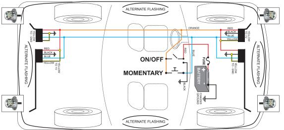
The front and rear heads are configured to flash independently of each other. In order to have the front and rear heads flash in sychronization, the blue wires from all units must be connected. The yellow wire can then be used to determine either alternate or simultaneous flash between each unit in the system by connecting to either power or ground.
