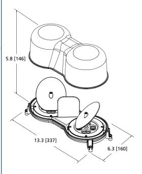
45° angled reflector driven by a quiet brushless magnetic drive system provides an exceptional warning beam without compromising reliability
