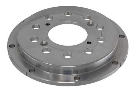
The mounting bells used in EBC Brakes Racing's 2-piece rotors are each precision machined from a billet of aerospace grade aluminium, ensuring they are both strong and lightweight. The bells are subsequently black anodised, providing an aesthetically pleasing and corrosion-resistant finish, allowing the mounting bells to be re-used for multiple outer friction rings thus leading to lower long-term running costs.
