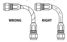
Do not twist during installation. This can be determined by the printed layline on the hose. Pressure applied to a twisted hose can cause hose failure or loosening of connections.
