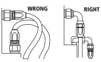
Use elbows and adapters in the installation to relieve strain on the assembly and to provide easier and neater installation that are accessible for inspection and maintenance.
