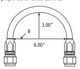
Minimum bend radius is measured on the inside bend of the hose. To determine minimum bend, divide the total distance between ends (B length) by 2. For example, B=6, minimum bend radius=3.
