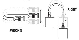
Make sure relative motion of the machine components produces bending rather than twisting of the hose. Hose should be routed so that the flex is in the same plane as the equipment movement.
