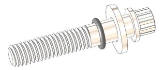
2. Install the large and small O-rings into their respectable locations on the adapter.
