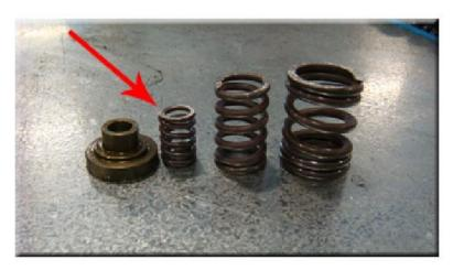
This photo displays 3 governor springs. The *smallest* spring (indicated by the red arrow above) should <u>NOT</u> be used with the 160hp, 175hp or 180hp pumps. *Without* the small spring installed, you should expect 3,000 - 3,200 rpm engine free rev. *With* the small spring installed, expect about 4,000 rpm engine free rev.
