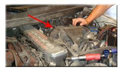
2. Unplug pigtail from the fuel shutoff solenoid.
