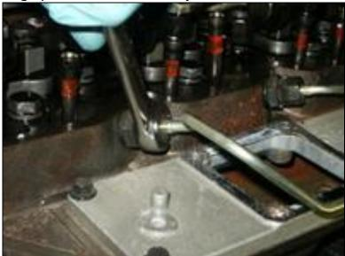
13. Loosen 13mm bolts on back of head that hold bracket just behind last injector line.
