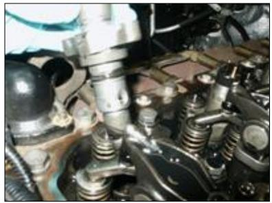
31. Insert connector tubes into place, balls up. Make sure they click into place.
