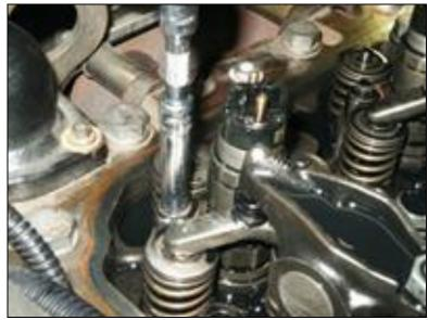
23. Carefully pry injectors out of injector bore.
