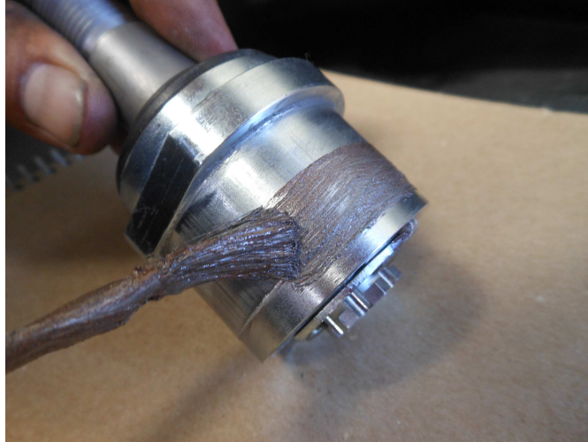
Figure 3, Applying Anti Seize to ProSteer Body
