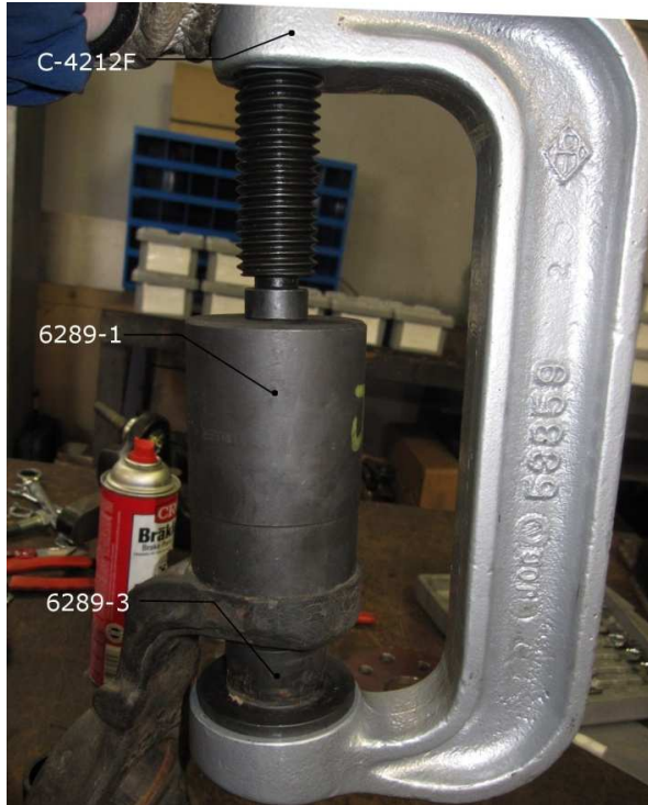
Figure 1, Upper Ball Joint Removal
