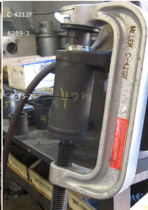
Figure 2, Lower Ball Joint Removal
