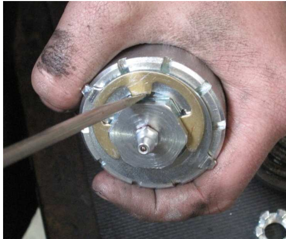
(Figure 7, Removing E-Clip Form ProSteer Upper Ball Joint) (Figure 8, Installing ProSteer Upper Ball Joint)
