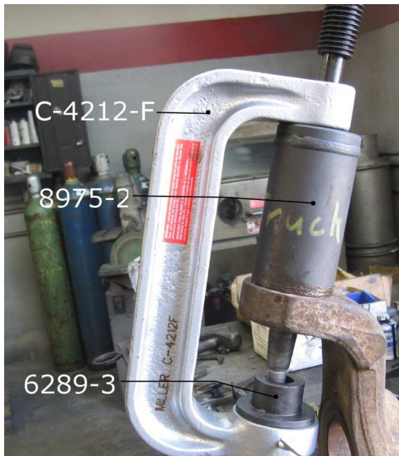
Figure 2, Pressing out Upper Ball Joint
