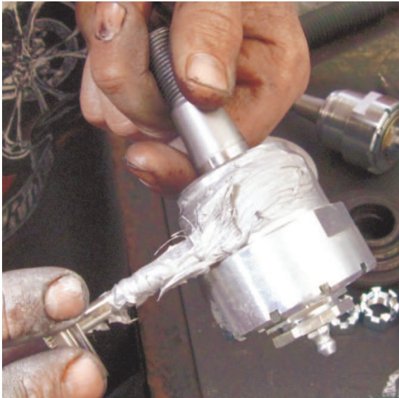
Figure 4, Applying Anti-Seize to ProSteer Body
