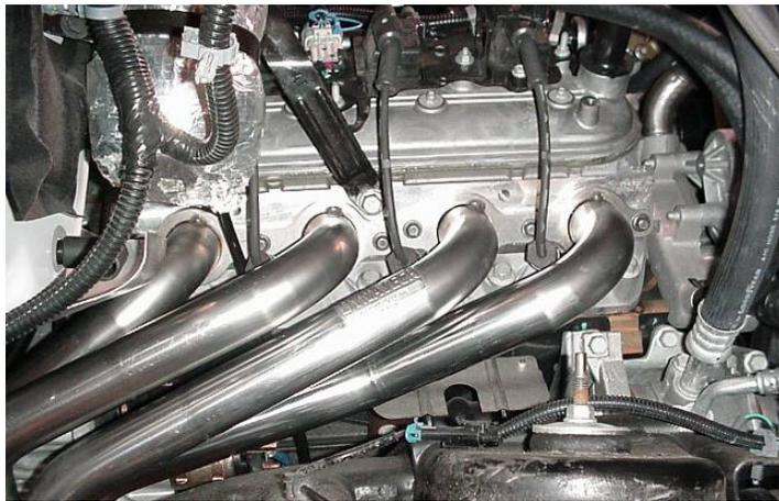
28) Reinstall any spark plugs that were removed and connect the wires to both the spark plugs and the coil packs.
