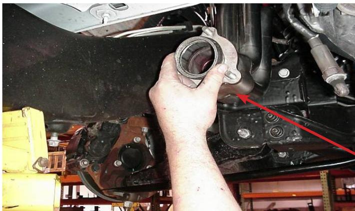
Install sintered donut gaskets before Y-pipe.
