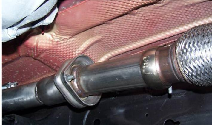
25) Driver's side catalytic converter & pipe can now be slipped into right hand pipe and attached to header collector with 3 flanged nuts. Make sure band clamp is installed over pipe before slipping left and right of "Y" together.
