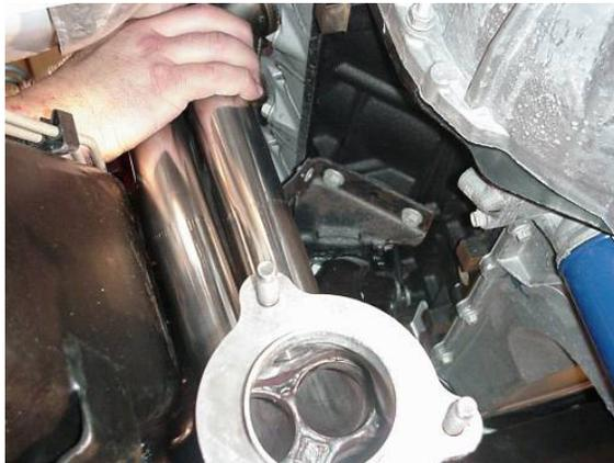
20) After installing both headers and all header bolts, brace transmission in the same manner as done in removal of stock "Y" -pipe.
