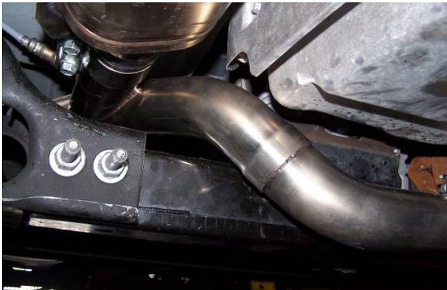
Use the single bolt band clamp to connect the catalytic converter to the "Y-Pipe".
