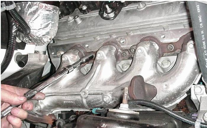
Use caution when last manifold bolt is removed as not to drop manifold.
