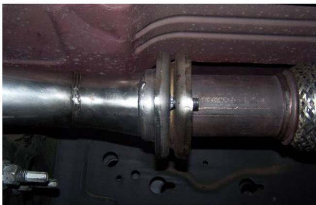
Stock cat-back section must be gently pushed back to accept new Y-pipe.
