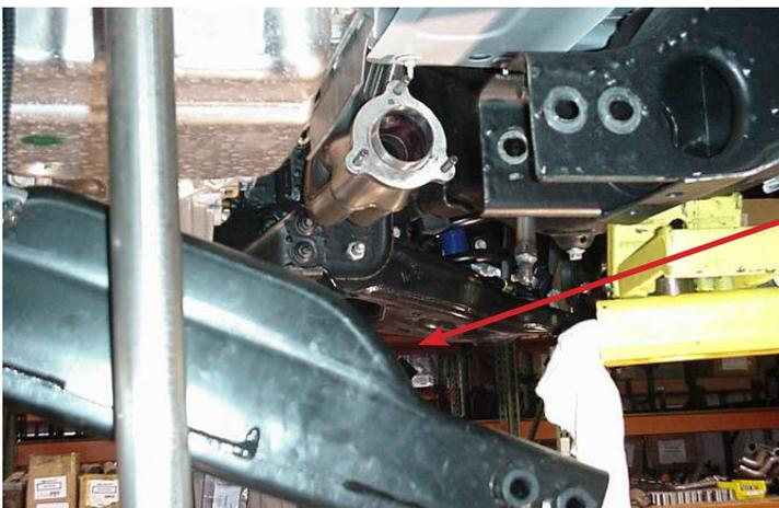
Here is the cross member lowered for removal and install.
