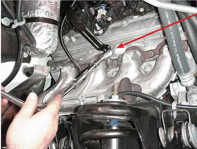
Remove dip stick tube retaining bolt, using care not to damage the “O” ring on the dip stick tube.
