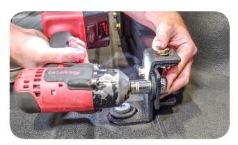
STEP 16: Now insert the tire screw mount and rotate so it sets in place vertically... see photos.
