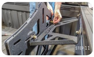
STEP 12: Next if the carrier is in its desired place...start at the side bed rail and tighten the 13mm hardware.
