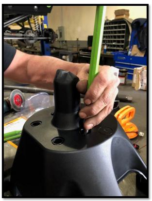
14. If using a camera, place factory camera mount and camera (plastic) though holes. Place factory stud plate behind it. Secure using factory screws.
