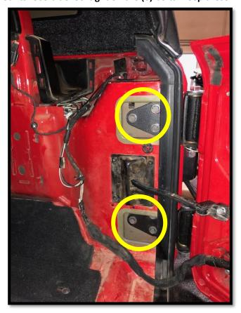
7. Install the new carrier onto the hinges. Using the included delrin bushings and stainless sleeves, slide the carrier into the hinges and secure with provided bolts and washers.
