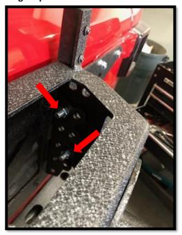
18. Tighten down (4) four tire mount bolts. Ensure all hardware is secure. Install plastic bumps on side of carrier. Plug in camera and third bracket light. Attach tire and test door.
