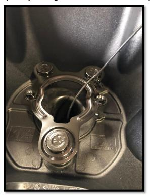
13. Using a punch, lightly tap out the factory camera mount. NOTE: This is plastic and so be careful and punch out the two holes in the center equally.
