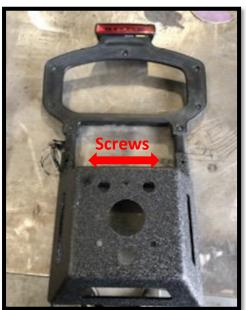
11. If you are running a rear camera you will utilize the factory camera bracket (plastic) and the provided camera enclosure. If you do not have a camera, you will utilize the block off plate.
