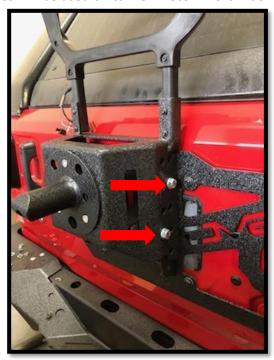
17. On each side of the carrier, place one bolt at the highest point on one row of holes, and one at the lowest point of connection with the tailgate plate and tire mount on the other row.
