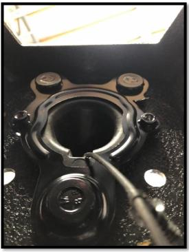
15. Using the provided camera enclosure, cover the camera and bolt using supplied flush mount allen head bolts.
