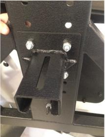
19) Place the final piece of the tire carrier into the slot shown below and use the two bolts provided to loosely attach it.
