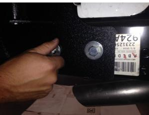
12) Ensure that the bumper is level. If it is not level repeat steps 12-15 making adjustments to level the bumper. NOTE: If the bumper is not level have a friend hold it level and tighten the side bolts first and then tighten the rear cross-member bolts. The bumper should be mounted as level as possible.
