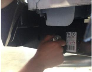
10) Next tighten the four center bolts in the rear cross-member first to allow the bumper to properly align itself. Torque to 60 ft/lbs.
