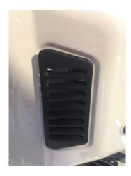
3) Once the vent is off, locate the small wiring harness just inside the vent and unclip it. This is the wire to the factory third brake light.
