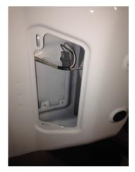
4) Next, remove the rubber plug and wire from the tailgate that is connected to your rear brake light. The plug should pull through if you disconnected the wires correctly. If it is not
