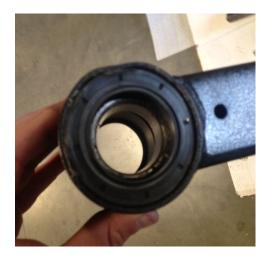
16) Carefully place the carrier back on the shaft with small bearing on top. Now add the fat washer before the castle nut. Tighten castle nut until it stops abruptly again and back off nut just far enough to get the cotter pin thru the hole in the shaft. NOTE: If you don't have enough room for cotter pin, that is a sign that you need to press the bearing race in a bit more. Simply put a little more torque on the castle nut and you will be able to press it in more.
