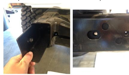
7) Next insert the 4 large 3"x 12mm through bolts through the frame rail with the threads facing the rear of the Jeep, make sure to put the washers onto the bolts as well. NOTE: You'll have to put the head of the bolt above the exhaust canister to get it into the hole.
