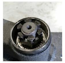
15) Next step is packing the bearings with grease. Once bearing is packed, turn the carrier upside down and place the large bearing in the bottom of the carrier, small side first. Next, install the seal over the bearing by tapping the seal in with piece of wood across it and a rubber mallet. NOTE: It's ok if peels away a little rubber off of the seal when tapping it in.
