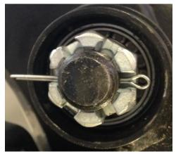
17)Bend the end of cotter pin to secure. Set the cap onto the whole assemble with the holes lined up that are highlighted below and then insert the small tapered head screw and tighten.
