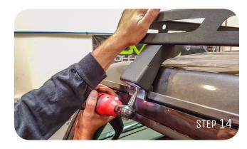
the top, tighten the gutter mounts 10mm socket or wrench on the top
