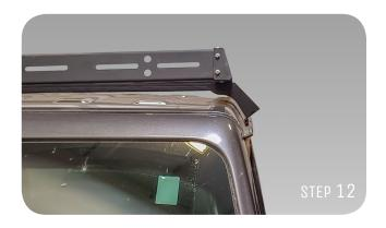
STEP 13: Next install the gutter clamps on each mount using the 2 H4 hardware screws.
