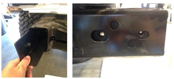
3) Next insert the 4 large 3"x 12mm through bolts through the frame rail with the threads facing the rear of the Jeep, make sure to put the washers onto the bolts as well. (You'll have to put the head of the bolt above the exhaust canister but to get it into the hole but it will fit)
