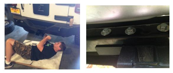
7) Then tighten the 4 side bolts that are loosely inserted into the nut plates. Torque to 60 ft/
