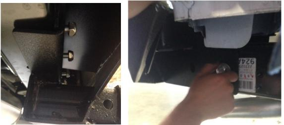
6) Next tighten the through bolts in the rear cross-member first to allow the bumper to properly align itself. Torque to 60 ft/lbs.
