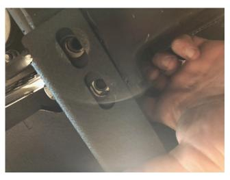
17) Hold the bumper up to where the OEM bumper was mounted. The two frame rail brackets will slide over the frame as shown in the illustration below.
