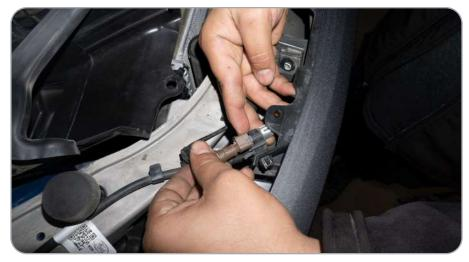
b. Black Washer Connecter: Squeeze the two sides together and firmly pull apart.
