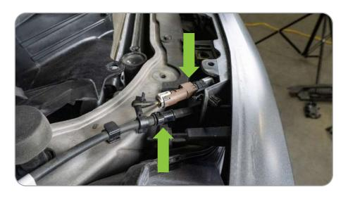
a. Brown Plug for Camera: Push the clip on the top and pull the two parts away from each other.
