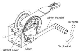
lose small parts. Turn the lever over and reassemble. Do not over tighten bolt. Check operation to insure the ratchet lever rotates fully without binding.
